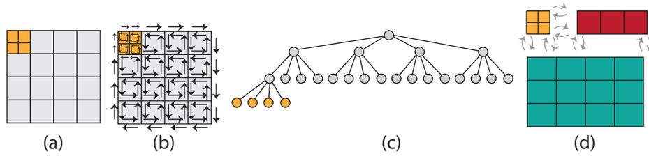
**Fig. 16.** (a)  $f \in CM(i)$  is subdivided. (b) Half-edge pointers needed for edges of the patch in (a). (c) Pointers needed to store the patch in (a). (d) Adaptive ACM and its essential connectivity information.
