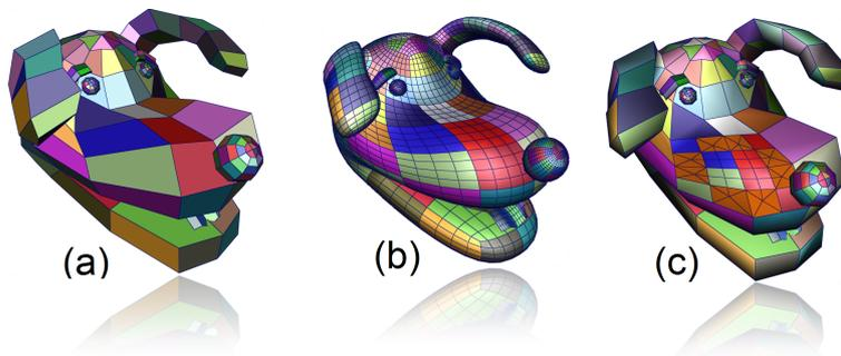
**Fig. 1.** (a) Coarse model. (b) A semiregular model obtained by uniformly subdividing the coarse model in (a). (c) Adaptively subdividing regions of interest. Patches at different resolutions are connected by zippers highlighted with orange faces.
