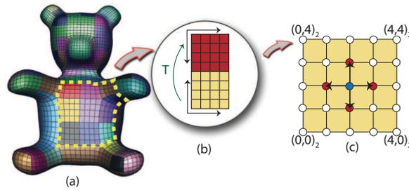
**Fig. 2.** (a) A semiregular mesh. (b) For each patch, a 2D domain (connectivity map) with a coordinate system is assigned. To move from one patch to another, a transformation between the coordinate systems of two adjacent connectivity maps can be used. (c) To index vertices, the coordinate system defined for each patch is used. The subscript of the index refers to the resolution of the refinement. Neighborhood vectors are used to obtain neighbors of internal vertices.
