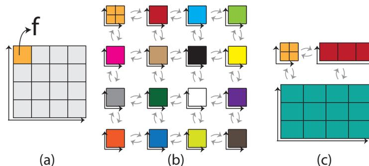
**Fig. 5.** (a) Face  $f \in CM(i)$  is supposed to be subdivided, therefore  $CM(i)$  has to be split. (b) Simple and inefficient solution for splitting  $CM(i)$  by assigning a connectivity map to each face. (c) A more efficient split of  $CM(i)$  that benefits from the regularity of  $CM(i)$ .
