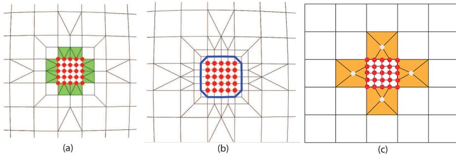
**Fig. 17.** (a) Red-green rule. (b) Incremental adaptive subdivision. (c) Zippers in the adaptive ACM. Images (a) and (b) are taken from [20, 19].
