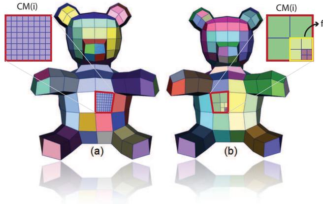
**Fig. 4.** (a) Adaptive subdivision with patches at different resolutions. (b) Adaptive subdivision with faces in a patch at different resolutions.
