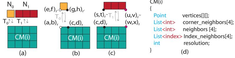
**Fig. 7.** (a)  $CM(i)$  is connected to two connectivity maps  $N_0$  and  $N_1$ . Transformations  $T_0$  and  $T_1$  are necessary to traverse these neighbors. (b), (c) The transformations that map a vertex in  $CM(i)$  to its neighbors are determined by storing necessary indices from the neighboring connectivity maps. (d) The new structure of the ACM.
