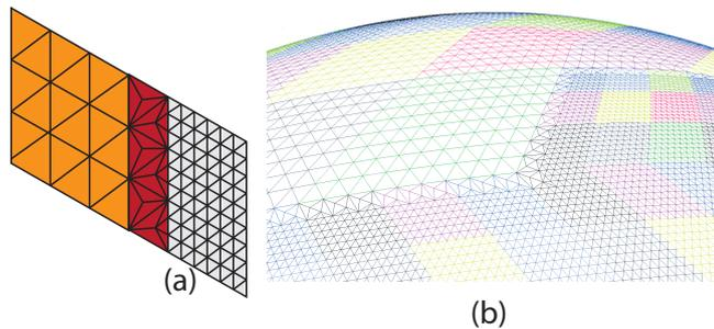
**Fig. 11.** (a) Zipper between two triangular connectivity maps. (b) Connectivity maps and zippers on a portion of the Earth.
