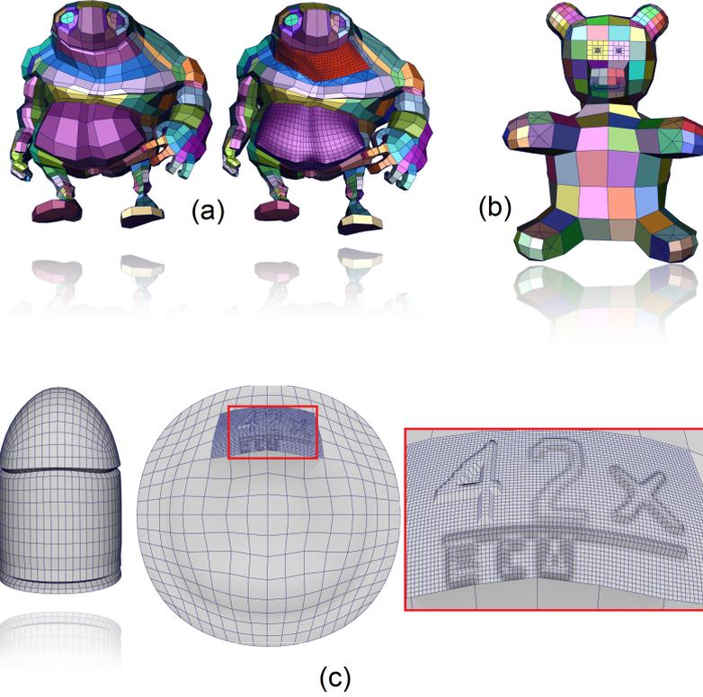
**Fig. 15.** (a) The Big Guy is adaptively subdivided on its belly and neck. Fine faces resulting from adaptively subdividing two different connectivity maps on its neck (purple and blue) are merged into a single connectivity map (red). (b) The hands and legs of Teddy are adaptively smoothed and some low scale details are added to the lips and the eyes of using adaptive refinement and local vertex manipulation. (c) The caliber of the Bullet is engraved on its back using adaptive refinement.
