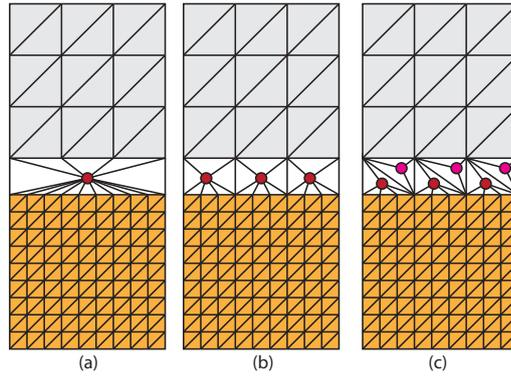
**Fig. 10.** (a) A zipper with one high valence vertex produces poor triangles (b) Adding more vertices to the zippers produces better triangulations. (c) It is possible to add vertices and retriangulate the zipper in (b) to achieve a better transition from a high resolution connectivity map to a low resolution one.
