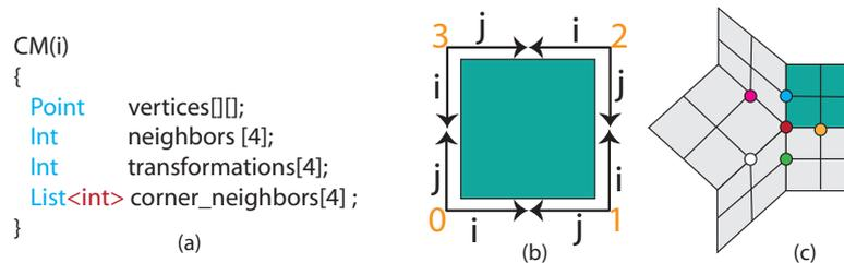
**Fig. 3.** (a) The elements that are stored for each connectivity map. (b) Inter-patch transformations are encoded as integer numbers. (c) A corner (red vertex) can be extraordinary. Connectivity maps attached to corners (in this case, two of them) are saved in `corner_neighbors`.
