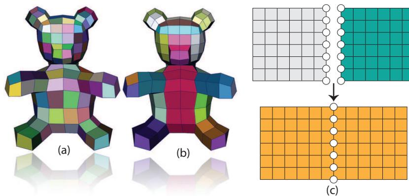
**Fig. 12.** (a) The original ACM, where a connectivity map is assigned to each individual quad at the first resolution. (b) Adaptive ACM supports larger initial connectivity maps. (c) When two connectivity maps are combined, duplicated vertices are discarded.
