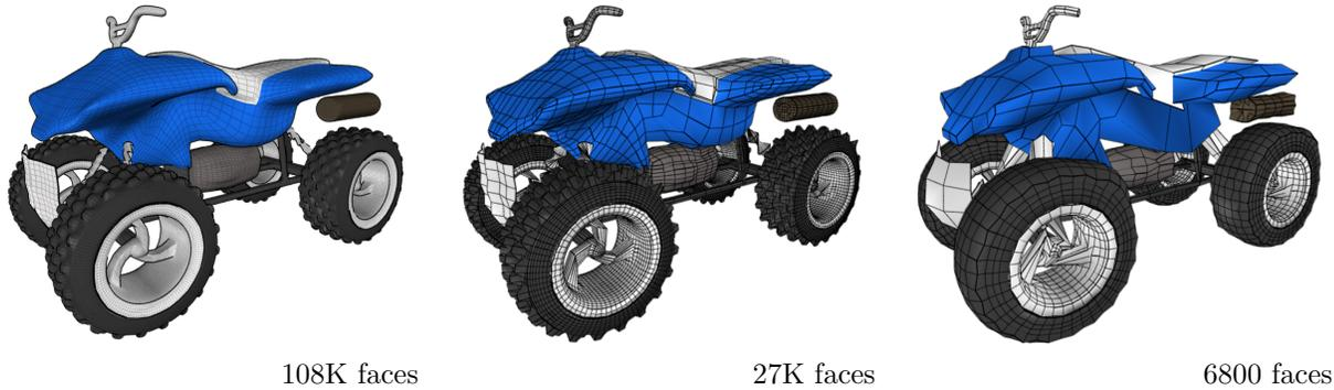
**Figure 12.** Decomposition of a complex surface: with only 1/16th of the geometric detail, the rightmost surface is a faithful representation of the original.
