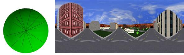
Fig. 4. A spherical panoramic projection surface (left) and projected image (right). The blue lines within the surface indicate rays used that might be used to a column of the image.
