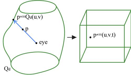
Fig. 10. When rasterizing we transform  $p$  from camera coordinates  $(x, y, z)$  to parameterized volume coordinates  $(u, v, t)$ . We can find  $(u, v)$  quickly by identifying the ray (with unique spherical coordinates) that passes through the eye,  $p$ , and  $p^*$  as shown on the left. On the right we produce interpret and rescale the volume parameters  $(u, v, t)$  as existing in the normalized device coordinate viewbox.
