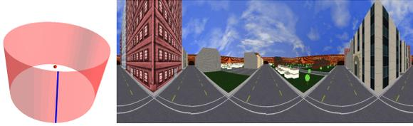
Fig. 2. A cylindrical panoramic projection surface with marked seam and center of projection (left) and projected image (right).
