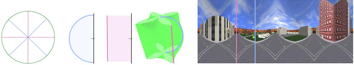
Fig. 8. An example of multiple profiles blended with linear interpolation. From left to right the images show the outline, the profiles, the surface and the panoramic image. The colored lines on the surface and image indicate positions where a single profile has influence.
