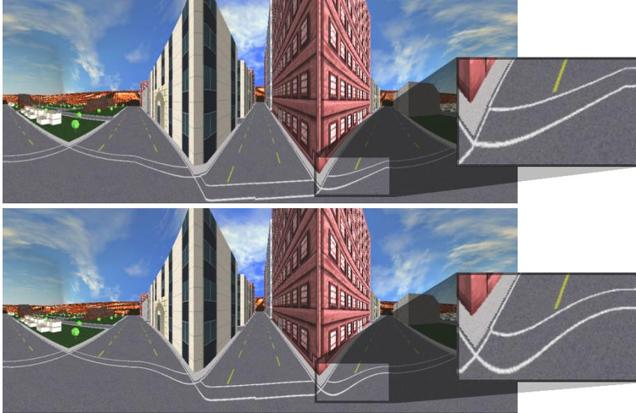
Fig. 9. Comparison between linear (top) and Bézier based (bottom) interpolation between profiles. Transitions between profiles are most noticeable in the magnified area examining the crosswalk lines. With linear interpolation the crosswalk lines transition sharply; Bézier interpolation creates a curved transition.
