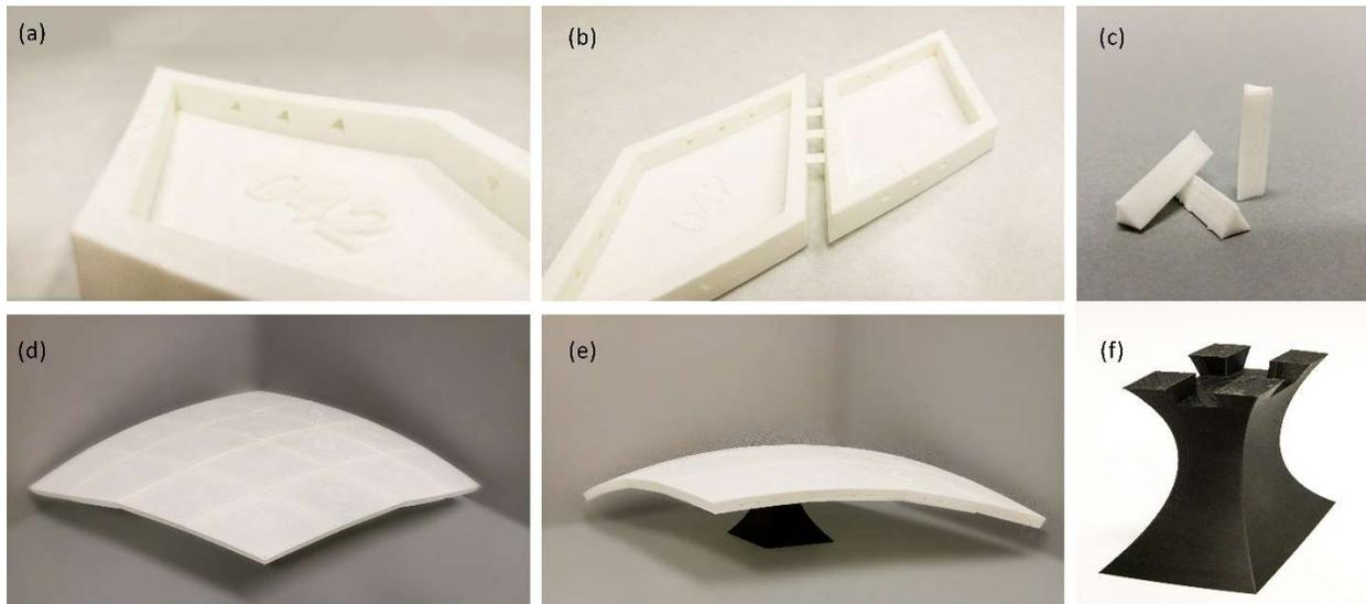
Figure 5. (a) The index of each diamond is engraved at its back. (b) Female connectors are made on the edge of diamonds. (c) Male connectors used to attach diamonds. (d) A curved model of the globe with no attached data from top view. (e) The curved model from side view. (f) Base of the curved model to hold the whole structure.
