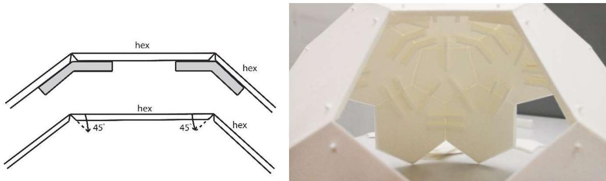
Figure 3. The designed connectors (on left) and the connected 3D printed faces (on right).
