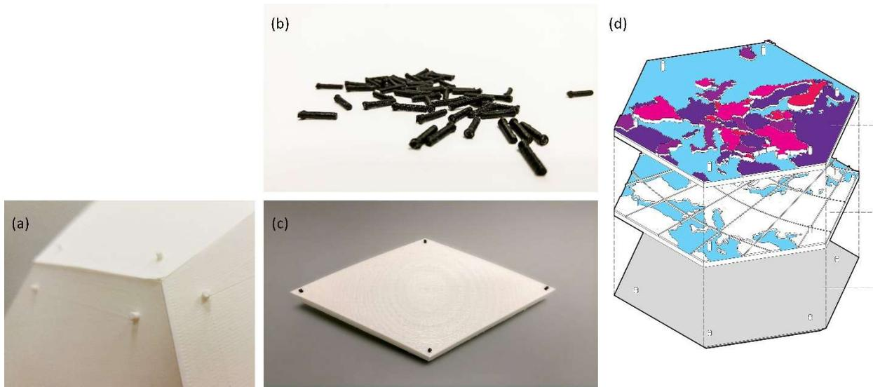
*Figure 6. On left, (a) pin-hole structure for the polyhedron globe. Middle: pin-hole structure for the curved globe. The pins (b) are inserted in holes carved into each diamond (c). On right, data layers to attach on cells. (d) The bottom layer is the main surface of the polyhedron globe. The middle layer is world political boundary data. The top layer is population data on a transparent paper.*
