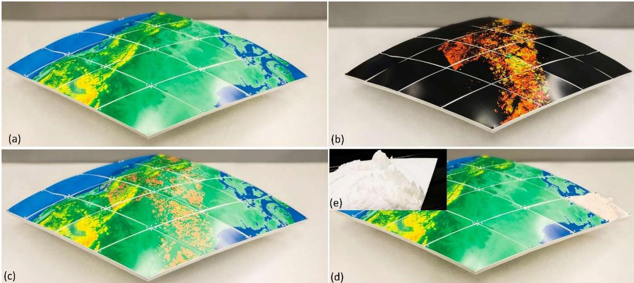
Figure 8. (a) Elevation data set of the western Canada attached to the 3D printed partial globe model. (b) Canadian National Fire data set. (c) The combination of the two data sets (Bottom). (d) A sample diamond containing 3D printed elevation data set.
