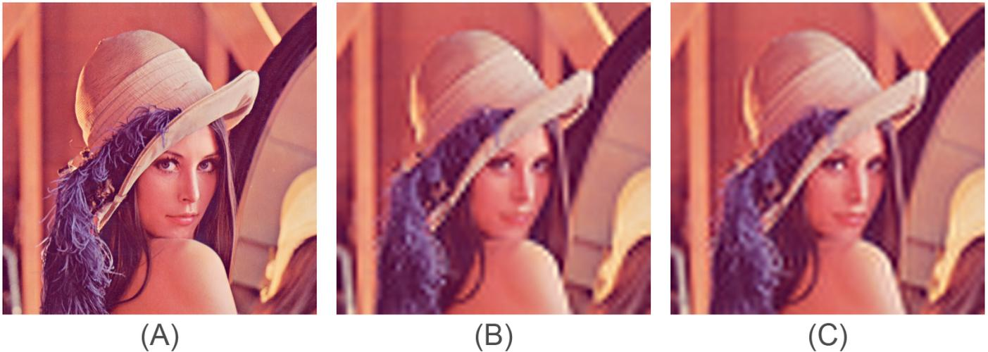
Figure 16: (A) The original Lena image obtained from [34]. (B) and (C) The results of compressing the Lena image using CDF9/7 and extended ( $l = 32$ ) interpolating CINPACT filters ( $c = 5, \sigma = 4.79$ ) respectively. Three decomposition steps are used. The PSNR value of luminosity is 25.3941 and 25.5484 respectively.
