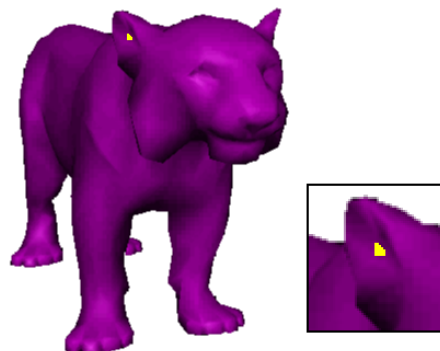
Figure 6: An active point can be used when the centre of the model doesn't provide an accurate enough depth. Here, the active point is on the left ear.
